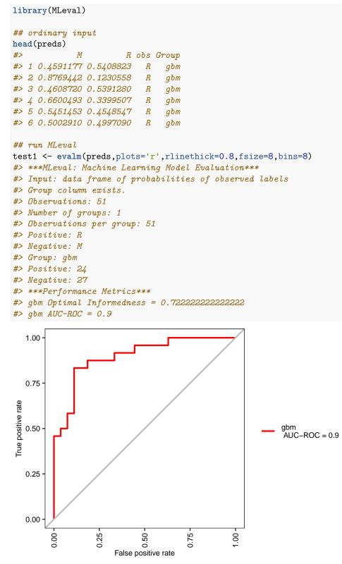
The ROC represents an ensemble of operating points corresponding to different probability cut-offs for
