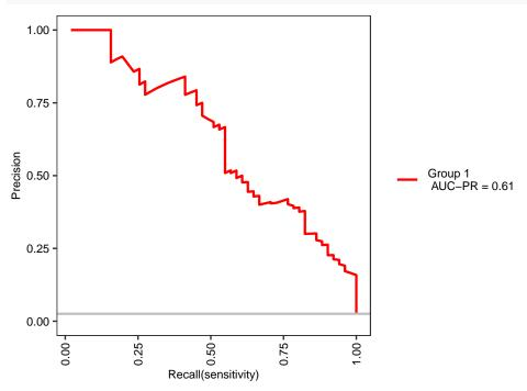
This is the precision-recall gain curve, which standardises precision against the baseline chance expectation. Flach and Meelis (2015) discuss in detail the preferable properties of precision-recall gain curves to precisionrecall curves. The precision-recall gain curve is telling us here our precision is quite poor relative to the baseline. Recall, the baseline for PRG curves is zero not a diagonal line like ROC.
