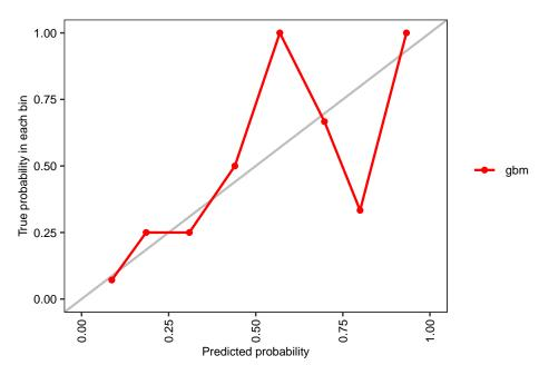
As we can see the calibration curve is quite similar to the idealised situation (diagonal line), therefore the model is fairly well calibrated. Calibration is an important part of determining whether a model produces sensible probability estimates, which is distinct from discrimination, i.e. ROC curve analysis.
